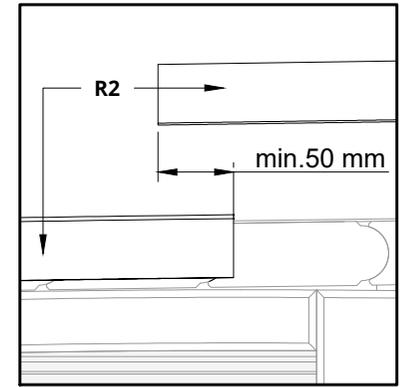
Install first outer underlayment so that the middle underlayment overlaps the outer ones by at least 50 mm to cover the nail heads.
