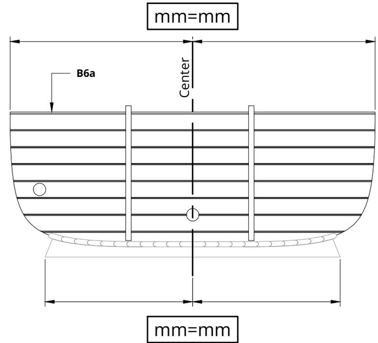
First install the lower part of the back wall. The lower part of the back wall must be in the center of the base.
