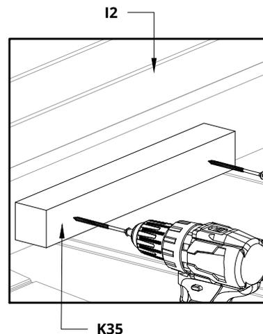
Next measure and install K55. Measure the top edge of the wall mount from wall mount K35 and install it against the back wall as shown in the picture.
