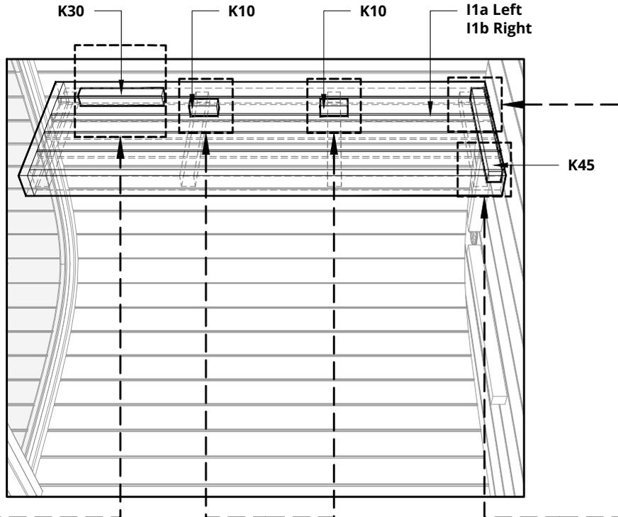
Install and fix the I1a upper bench to the wall mounts K45 with two S7 screws and K30 with two S5 screws.
