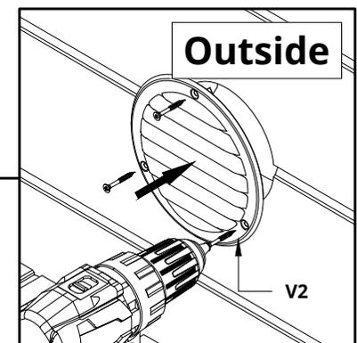
The inner and outer ventilation grilles V2 and adjustable cover V3 are screwed with 3 screws.
