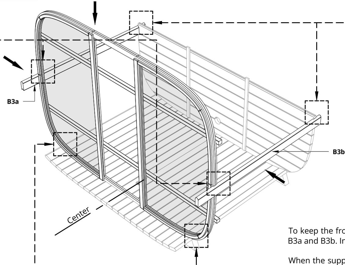
To keep the front wall upright, use the side wall boards B3a and B3b. Install them as shown in the picture.
