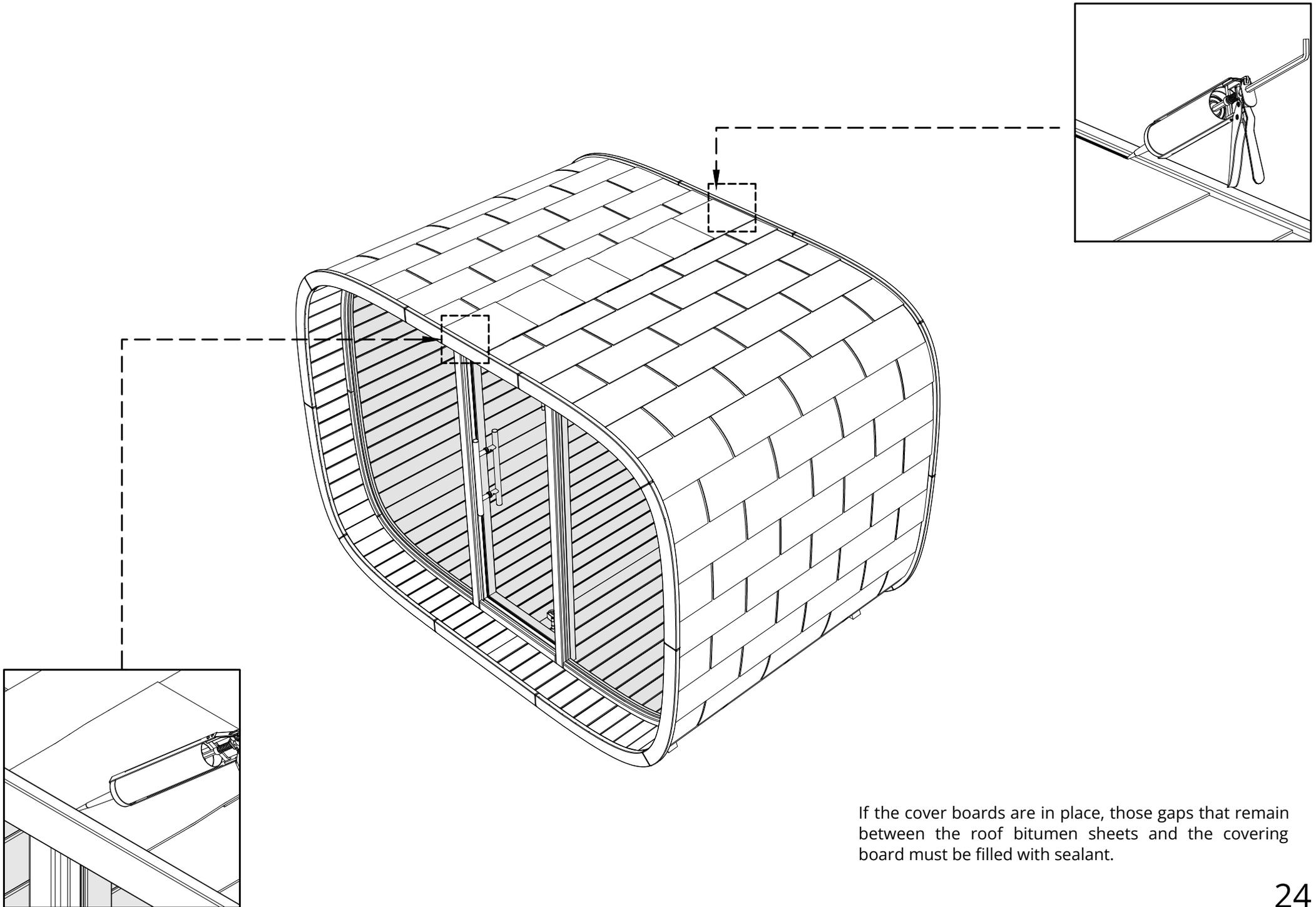
If the cover boards are in place, those gaps that remain between the roof bitumen sheets and the covering board must be filled with sealant.
