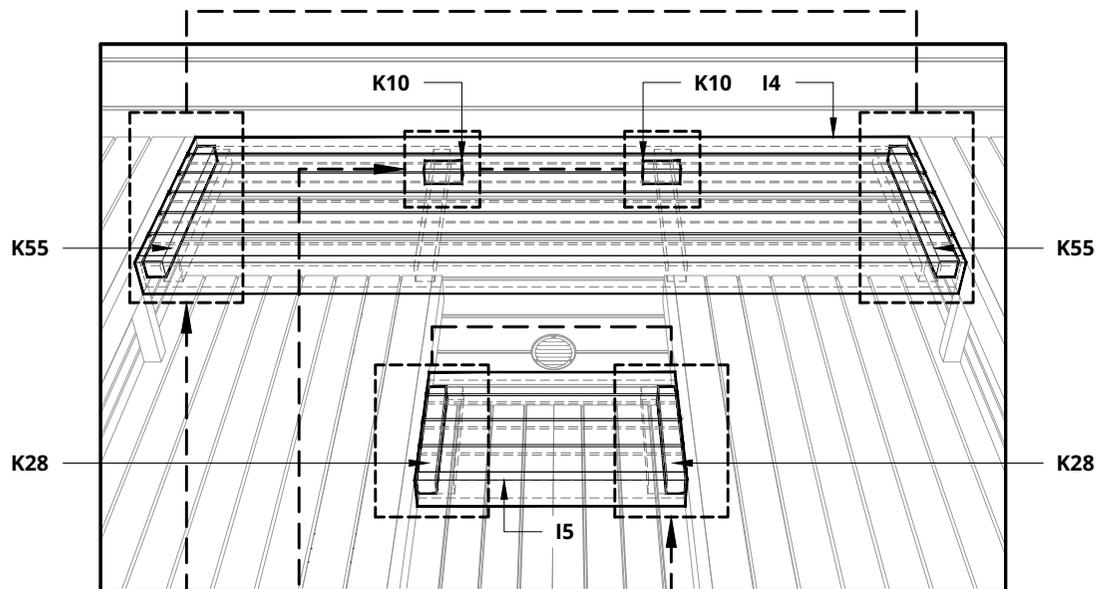
First install and fix the I4 upper bench to the K55 mounts with two screws.
