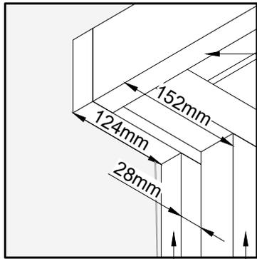
*The measurement must be started from the lower edge of the square wood attached under the bench for square wood legs.*
