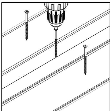
Insert the last piece and use a rubber mallet to tap the planks together. Screw the loose planks to the walls with screws.
