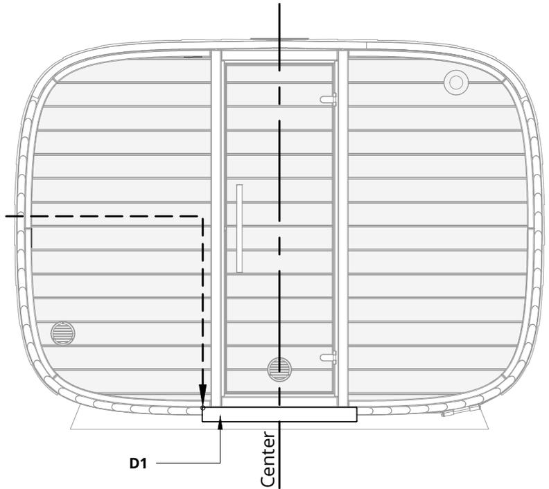
The installation of the cover boards is started from the bottom and the first cover board must be in the center at the front end and at the back end of the sauna.
