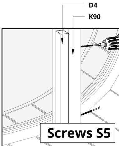
**The cover board is longer, it must be cut to the correct size. Height measurements are measured from a straight surface.**
