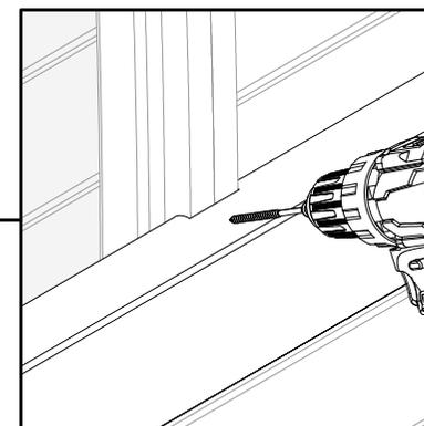
When the top of the back wall is in place, continue with the construction of the side walls. Use blanks B3a (left) and B3b (right) to build the side walls.
