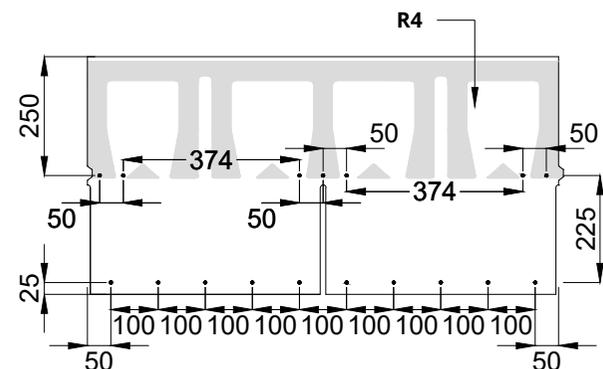
Remove the protective film from the bottom of the sheet and put it in place by starting the row from the bottom and center. The bottom edge of the first row sheet must be in line with the bottom edge of the base sheet shown in the pictures.
