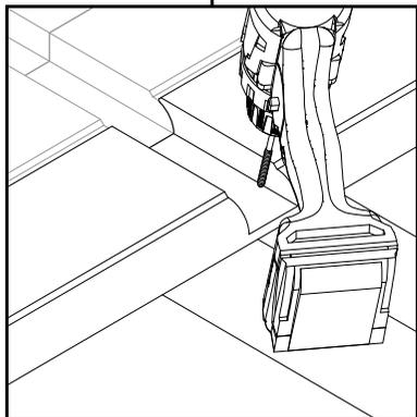
When the boards are installed it should look like this. ~10 boards on each side.
