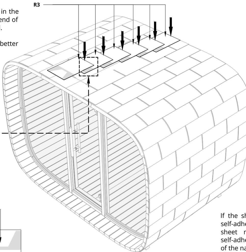
If the sheet is in place, fasten it with 4 nails on the self-adhesive spot as shown in the picture. The next sheet must be placed so that it overlaps the self-adhesive spot of the first sheet and covers the head of the nail min. length 150 mm.
