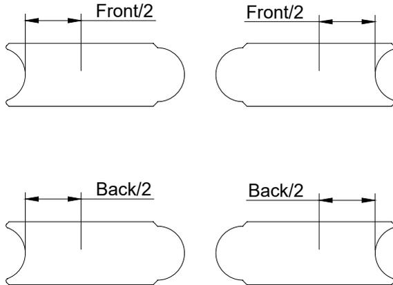
Divide the measurement by two and transfer the measurements to the last two planks. Connect the dimensions on the plank with a line and cut off these ends.
