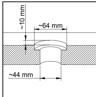
Before installation of the drain pipe, hole must be cut with a hole saw.
