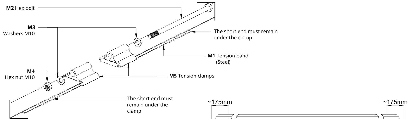
Place the tension bands M1 (Steel band) around the side walls and thread the bands into the eyelet as follows (see sketch above).
