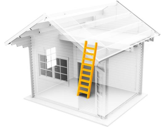
CONNECT THE OTHER HALF OF THE LADDER FITTINGS AND ATTACH THEM WITH SCREWS TO THE STAIRCASE.
