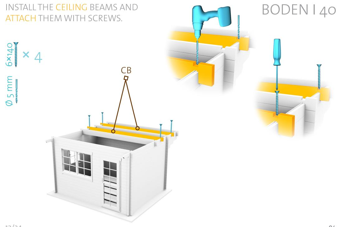
INSTALL THE BEAM AND BODEN 140 **ATTACH** WITH SCREWS. 53CW Ø4mm 5×70 BM
