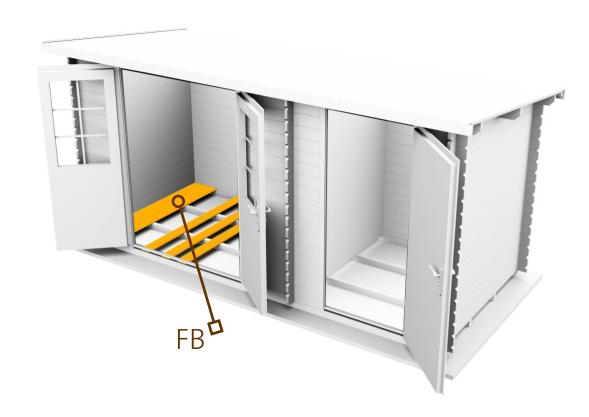
SAW THE BASEBOARDS AND ATTACH WITH NAILS AT EVERY 0,5 METERS.
